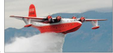
The Martin Mars is the largest flying boat ever flown operationally, with a height of 38 feet, a length of 120 feet, and a wingspan of 200 feet (approximately the wingspan of a Boeing 747). Only six of the massive aircraft were built in 1942 with the two remaining in existence used as water bombers on forest fires throughout the western United States, Canada, and Mexico.
